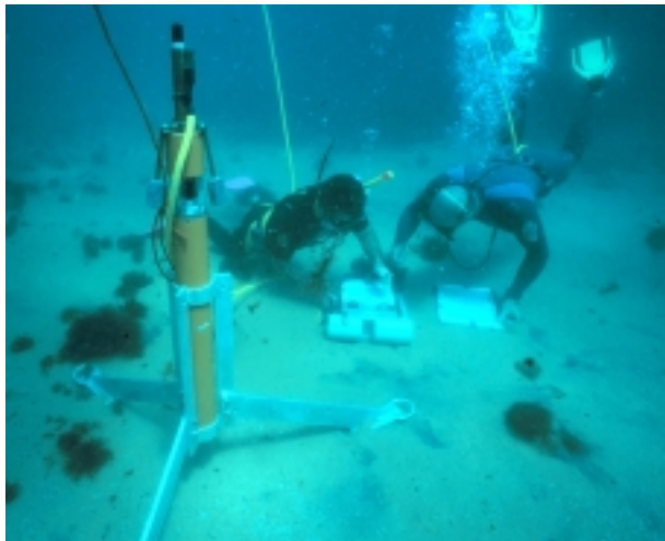
Figure 3. Calibrating a transponder, note the diver unit placed on top of the transponder.
